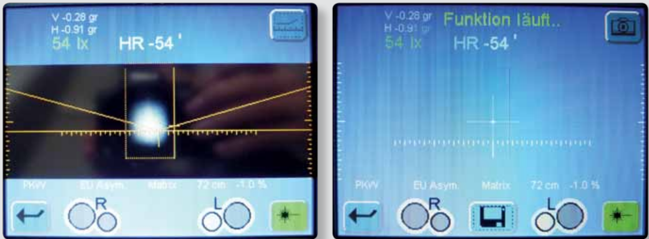
Adjustment of a headlight with Matrix LED technology (test image via ECU diagnosis right on the vehicle)
