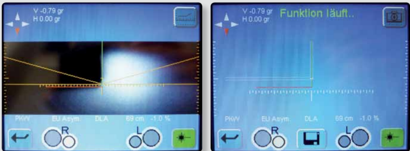
Adjustment of a headlight with DLA high-beam assistant (test image via ECU diagnosis right on the vehicle)
